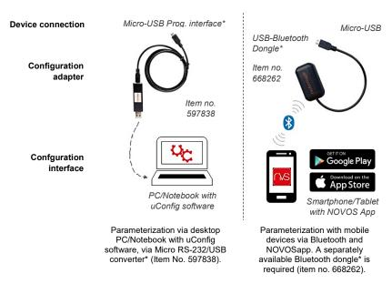
\*Commercially available Bluetooth dongles or USB to Micro-USB adapter cables are not compatible. You need a mobile device that supports at least Bluetooth version 4.1. The configuration app with the corresponding instructions can be downloaded from the Google Play Store or the Apple App Store.
