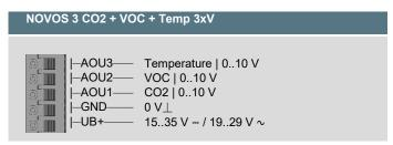
Room sensor CO2 + VOC + temperature + humidity - active 4x 0..10 V
